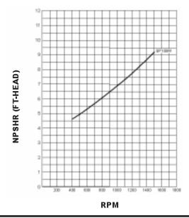
to the pump to prevent cavitation.
